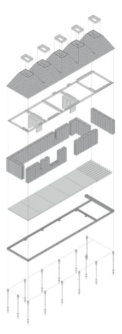
**Right**Site plan; exploded axonometric. The building has screw-pile foundations and a CLT deck, with CLT wardrobes to provide lateral stability to the cork block envelope.
